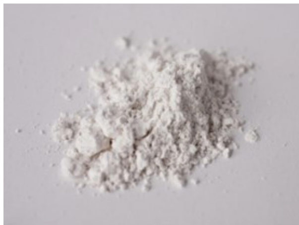
Figure 9. Lime used for making hempcrete Lime: https://www.lcgfrance.com/mortiers-et-enduits-isolants/ ; https://chanvra.org/pages/hemp-construction-materials-hempcrete ).
