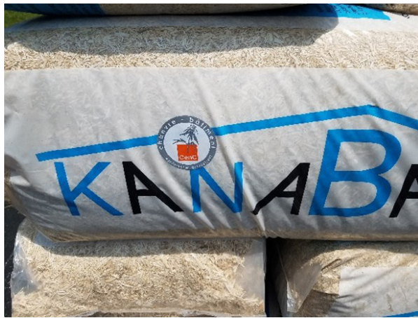
Figure 8. Hemp Hurd (Hemp: https://chanvra.org/pages/hemp-construction-materials-hempcrete ; A bulk sample of Kanabat Building Grade Hemp Hurd that can be used as alternative aggregate of hempcrete.
