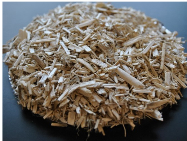
Figure 8. Hemp Hurd (Hemp: https://chanvra.org/pages/hemp-construction-materials-hempcrete ; A bulk sample of Kanabat Building Grade Hemp Hurd that can be used as alternative aggregate of hempcrete.
