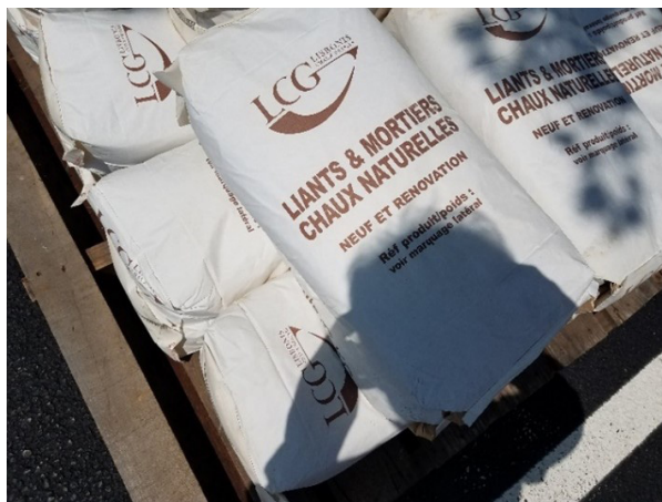
Figure 9. Lime used for making hempcrete Lime: https://www.lcgfrance.com/mortiers-et-enduits-isolants/ ; https://chanvra.org/pages/hemp-construction-materials-hempcrete ).
