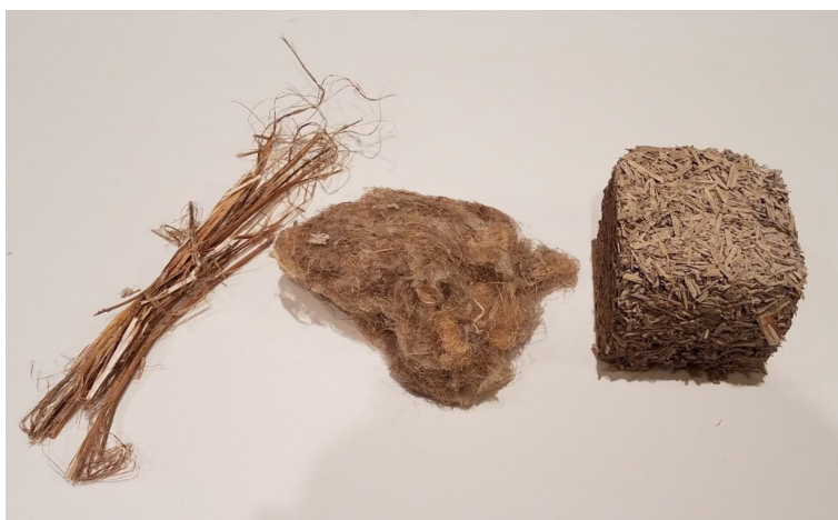
Figure 6. Example material used for retrofit: Hemp fiber and hard (left); Hempcrete block (right).
