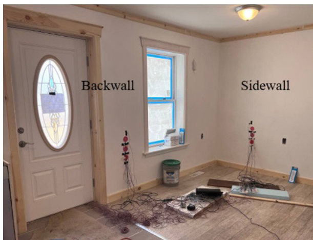
Figure 21. Positions of heat flux sensors on the side & back walls.
