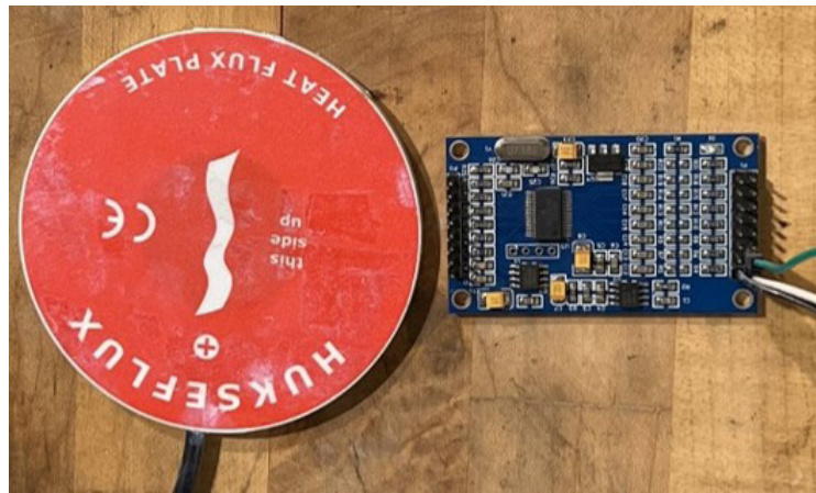
Figure 23. The connection of the heat flux to the ADC.
